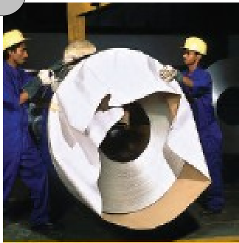
Strapping around the OD to hold the VCI paper & metal sheet on the coil
