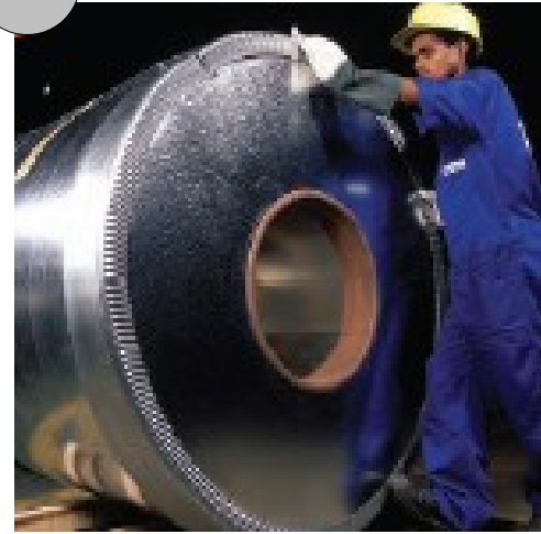
Fixing metal protectors on the sides and metal edge protectors on ID & OD straps
