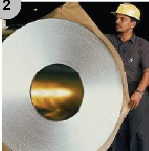
Placing the coil on HDPE fabric laminated VCI paper & metal sheet
