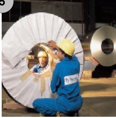
Tucking the VCI paper in to cover the edges and ID
