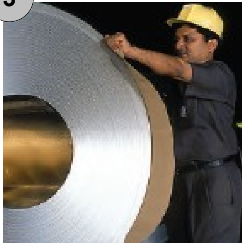
Wrapping the coil in HDPE Fabric Laminated VCI paper & metal sheet
